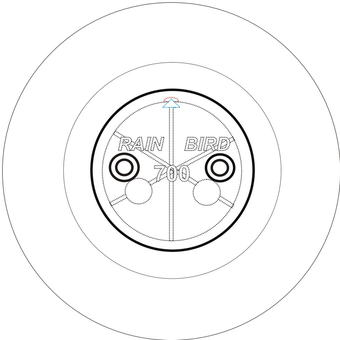
**NOTE:** Align notch (in red) on underneath side of yardage marker with arrow (in blue) on top of nozzle assembly
