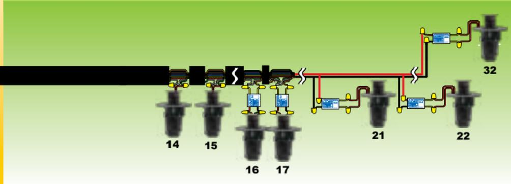
**USE "POWER" WIRES FROM EXISTING SPRINKLERS 16 & 17 FOR THE NEW 2WIRE PATH. BOTH SPRINKLERS NOW WILL BE OPERATED WITH A DECODER ON THE 2WIRE PATH BUT AS STATIONS 16 & 17**
