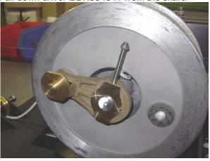
Cut cable so that the limit stop for Tracker™ (BTC584416 and ZK1484424) can be removed from the cable.
