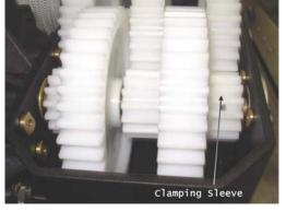
Apply blue Loctite Tracker™ shaft thread.
