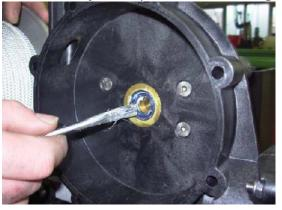
Check the assembled ball bearings for zero clearance and free movement in the gears & cover Tracker™ shaft. If necessary replace with a new deep-groove ball bearing (ZK1994372).
