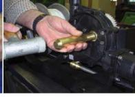
Lubricate rotary shaft lip seal with acid free grease (Molikode).
