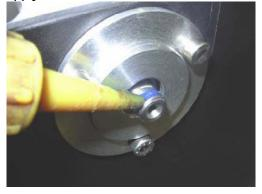
Unscrew nut clamp for Tracker™ shaft (BTA484370), attaching Tracker™ wheel with the left hand and tighten net with 9-10mm.
