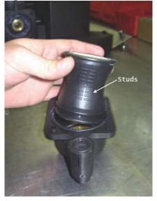
Re-assemble control module (1st spring, 2nd ball bearing, 3rd seal), as per detail X on the individual parts list.
