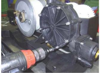
Re-assemble wheels, gear cover and cover to the unit.
