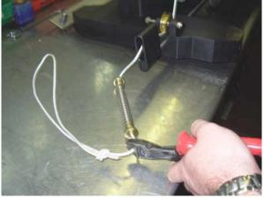
Remove cable drum from the shaft and replace with a new cable drum BB0284412.
