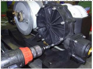
Attach Tracker™ wheel (BTV784312) with the left hand and remove screw (BTC484330) M10 to get to the Tracker™ shaft.
