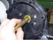
Insert new shaft seal (ZK0994377) with pressure bolt no. 3 (BTC584433) –
