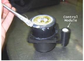
Replace valve casing using SW5 Allen key.
