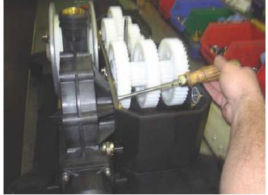
In case deep-groove ball bearing (ZK1994372) is intact: Tap out with pressure bolt No.1 (BTC584431) to gear case.
