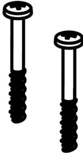
Use the screws from the Rain Bird rotor. Use o-rings between screw and Yardage marker
