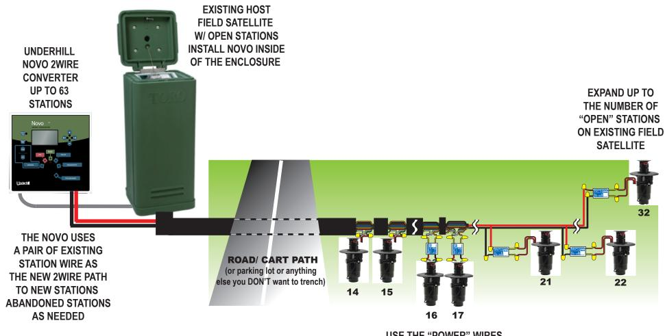
USE THE "POWER" WIRES FROM EXISTING STATIONS 16 & 17 AS THE NEW 2WIRE PATH. BOTH STATIONS WILL BE OPERATED W/ A DECODER ON THE 2WIRE PATH AS STATIONS 16 & 17
